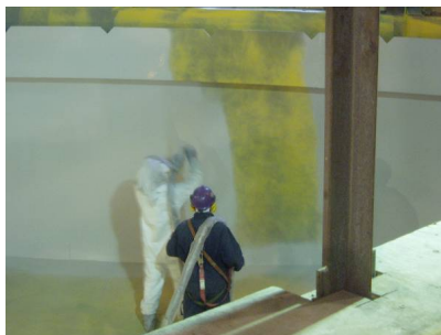
Leak testing of heat exchanger
