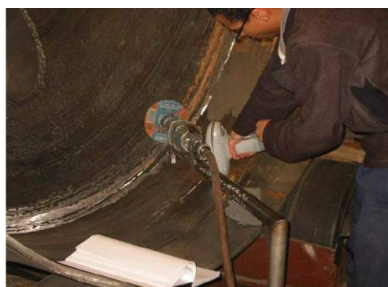
PMI of weld overlay with portable XRF analyzer
