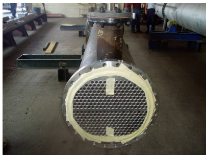
Leak testing of heat exchanger
