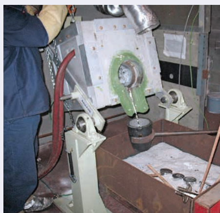
XPS Induction Furnace
