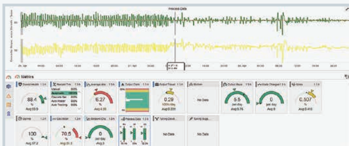
Figure 1: The oscillation on the left side of the marker - and operator work around on the right - had not been identified before CLPM was implemented.
