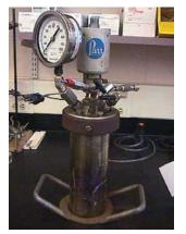
Pressure oxidation tests are carried out in a stirred 2L Parr bench-scale autoclave, which typically handles charges of approximately 1 kg. The autoclave is constructed of titanium and can be operated with an optional glass liner. It is fully automated to measure and control the temperature and pressure within the autoclave and the gas flow into the autoclave. The process
