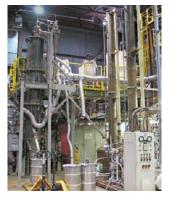
Comparative testing of all three options can be carried out at bench scale at XPS using the facilities and expertise on hand. Roasting can be completed in either 2", 4" or 12" diameter continuous fluid bed roasters, each equipped with a cyclone, afterburner for combustion of arsenic and/or sulphur vapour, condenser, and
