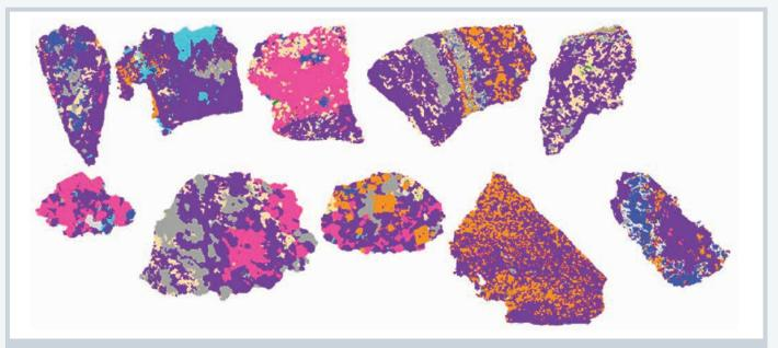
A zinc ore showing QEMSCAN images of sphalerite (purple) associated with galena (blue), pyrrhotite (pink), pyrite (orange), quartz (grey), carbonates (dark blue), orthoclase (cream).
