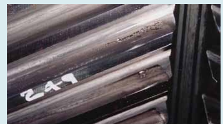
Progressive pitting damage on gear tooth face
