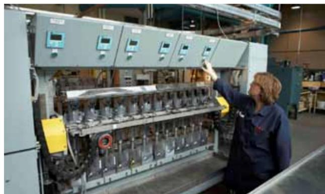
XPS Mini Pilot Plant (MPP) Flotation Unit
