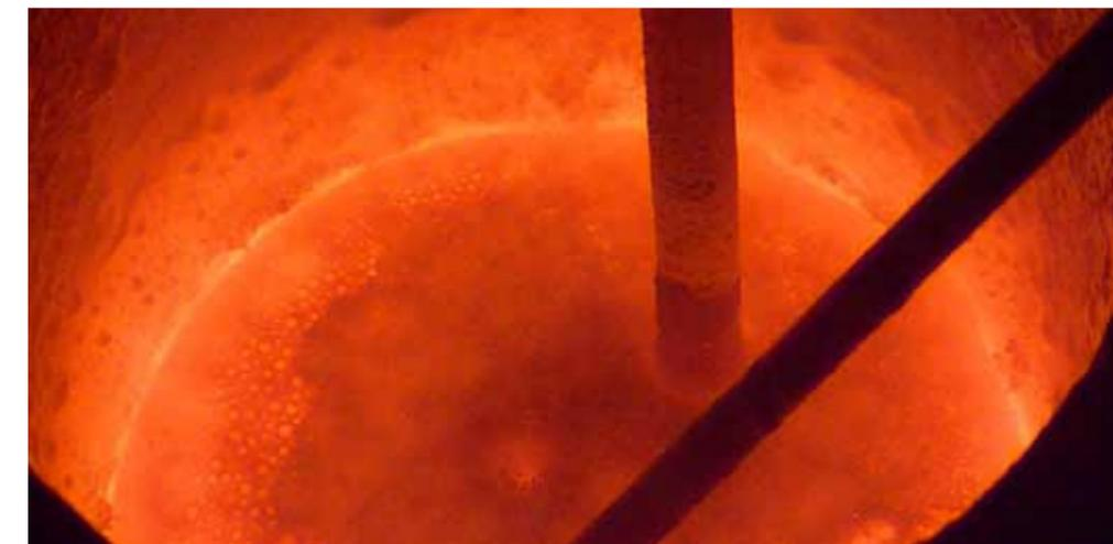
Smelting of EW residues in the induction furnace
