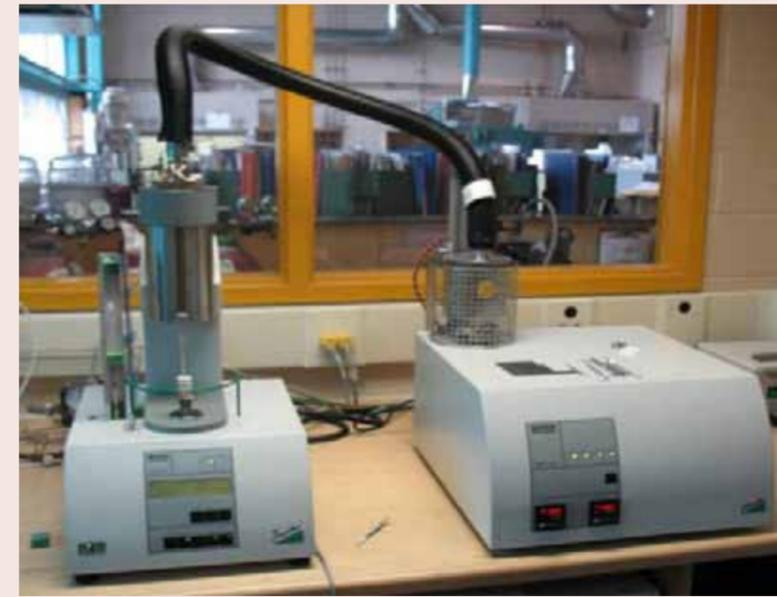
XPS Thermogravimetric Analyzer (TGA)
