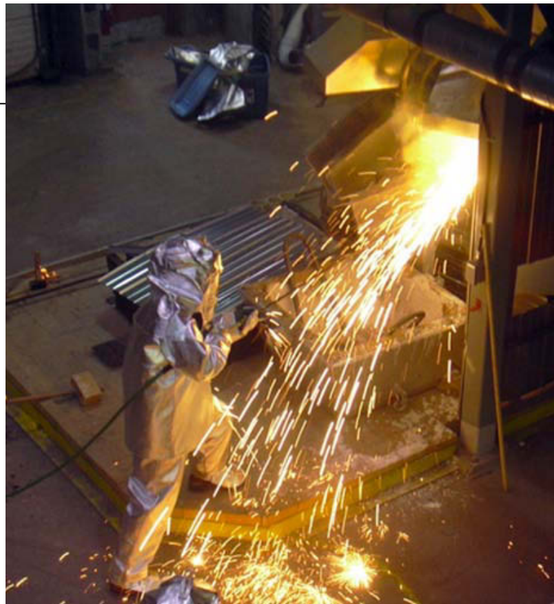
XPS employee tapping the DC arc furnace.
