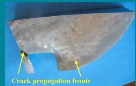
Figure 2: Fracture surface shows two crack propagation fronts
