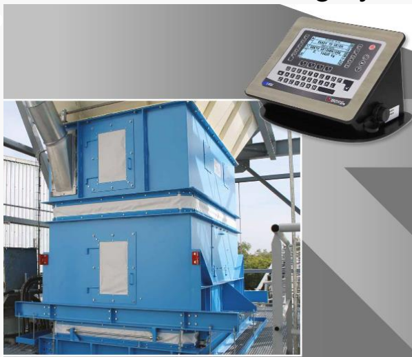
Discontinuous weighing – Hopper scales
